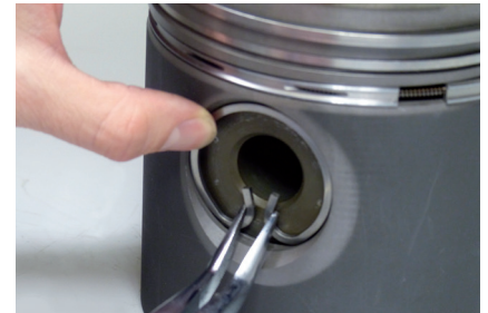
Figure 3: In this case, the ring opening should be at six o'clock or twelve o'clock
