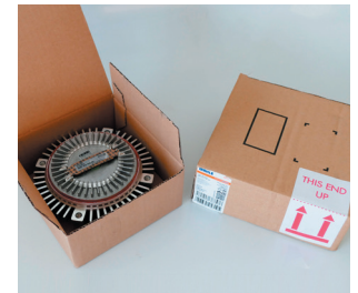
Figure 2: Correct storage position of a bimetallic Visco® clutch (according to packaging label with bimetallic strip facing upward)
