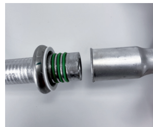
Figure 1: Separated spring-lock connection
