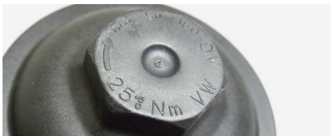
Figure 2: Torque specification on the housing cover
