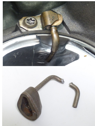
Figure 2: Cooling nozzle fitted (top) and broken off (bottom)
