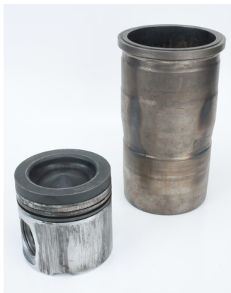
Figure 1: Overheated Ferrotherm piston (steel piston crown and aluminium skirt) showing seizing marks, with cylinder liner
