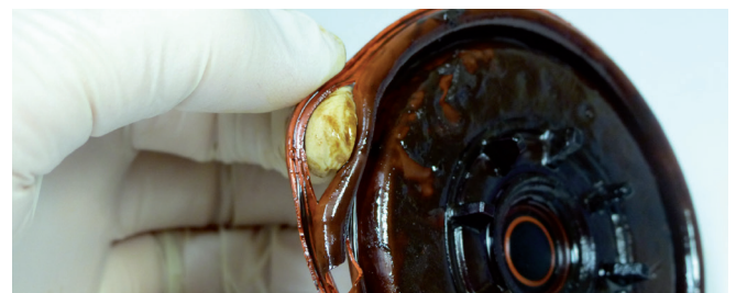
Figure 4: Cracked PCV diaphragm
