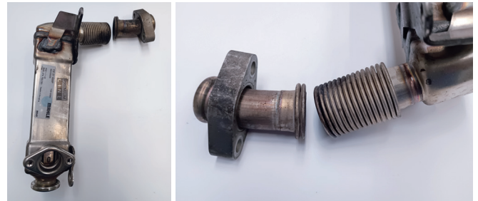
Figure 1: EGR cooler with cracked flexible pipe
