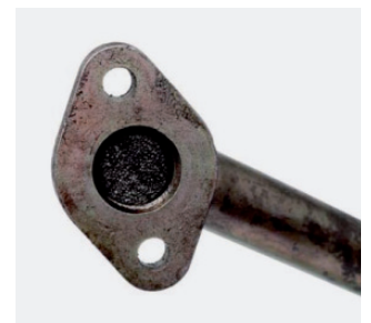
Figure 4: Carbonised oil return line
