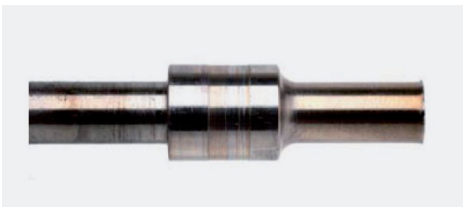
Figure 2: Clear signs of wear on the shaft at the bearing point
