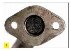
Additional causes include an overdue oil change, incorrectly installed oil pipe or a missing heat shield. Subsequent additional remedies include replacing the oil pipe and ensuring its correct installation and replacing the charge-air cooler and particulate filter if the turbocharger has been
