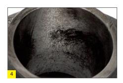
When it comes to the compressor wheel, stress is generally caused by dirty or an insufficient oil supply to the bearing, an increase in exhaust back pressure or a clogged air filter.
