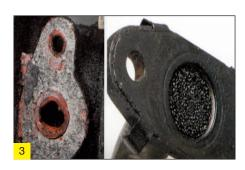
Probable causes include constriction or a bend in the oil return pipe, the use of sealing compound rather than a gasket set, the failure to replace the engine connection when replacing the return pipe, or even simply too much oil in the engine.
