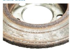
Score and groove marks on disc brakes
