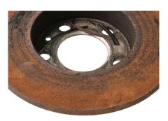
Severe rust formation on brake discs and pads.
