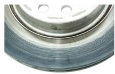
Brake pad fails to disengage and rubs against the disc. This can cause the brake system to overheat.
