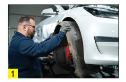
Step 1: Remove the wheel and inner wheel arch. Remove all clips and the screws located under the wing.
