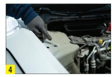
Step 4: Remove control arm top mount fixings, located in the frunk. The drain that allowed water to contaminate the original control arm is next to the mounts.
