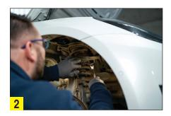
Step 2: Check all the other suspension parts for damage and general condition. Release the ABS wire where it is attached the control arm
