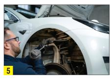
Step 5: Remove ball joint and control arm fixings. Pull the control arm out of the top mount.
