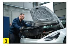
Step 3: Remove the frunk, by first removing the circuit breaker, and then the screws and clips.
