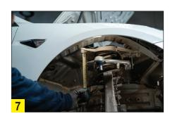
Step 7: Push the ball joint in the swivel bearing
