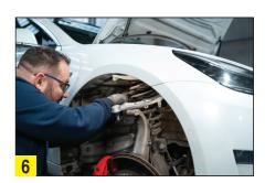
Step 6: Push the new MEYLE HD control arm into the top mount. Adjustment between the arm and the top mount should be 60mm.
