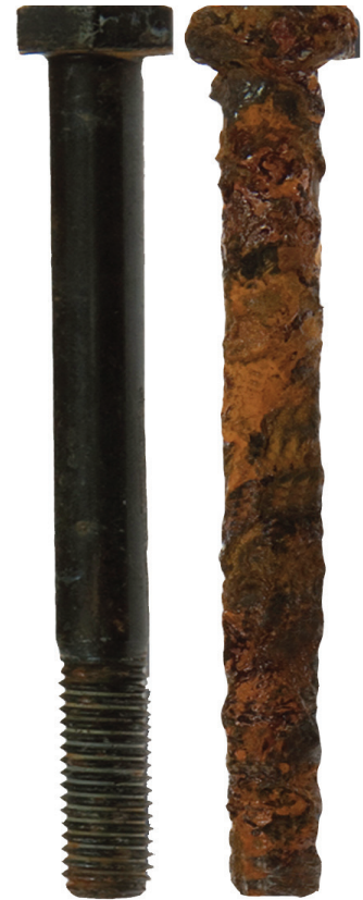
Meyle's zinc-nickel coated VAG replacement suspension bolt, at left, after a 480 hour salt spray edurance test. The other bolt is an OE suspension bolt, after the same test.
