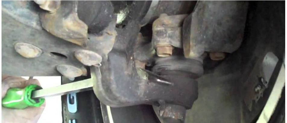
Use a pry bar to check ball joints and tie rod ends. Any free play is too much.
