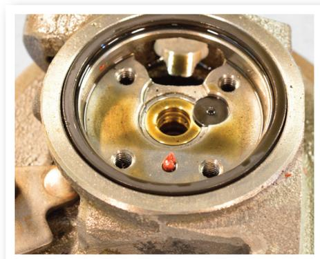
Sealant blocking the oil feed to the thrust bearing
