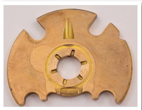
Scoring to the thrust bearing from a turbo that has not been primed
