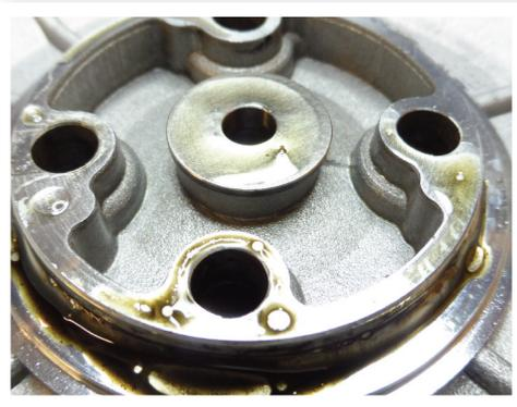
Coolant in the oil causes a 'droplet' effect as it separates
