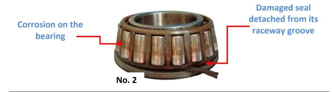
This failure is irreversible, the bearing and disc have to be replaced as a complete unit KF155.70U
