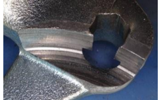
Abrasion mark caused by roller contact
