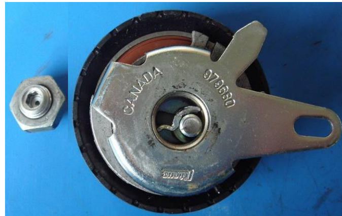
Roller GT357.28 with broken shaft
