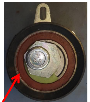
Roller GT357.28 with broken shaft
