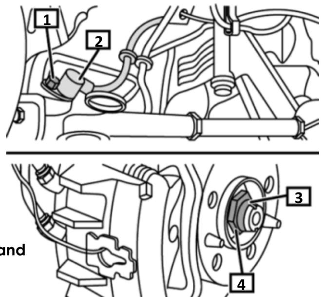
**8) Use a ball joint puller to remove the steering ball joint from the stub axle (no.5)**
