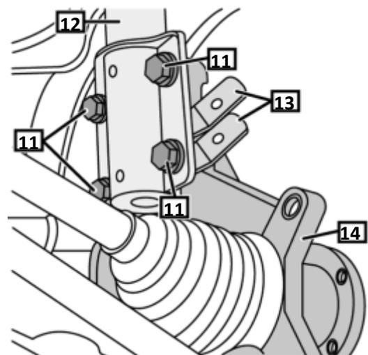
**12) Unscrew the bolts from the strut (no.11)**
