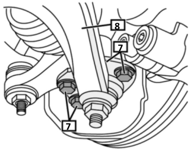
**9) Unscrew the bolts from the lower joint (no.7) to release the control arm (no.8)**
