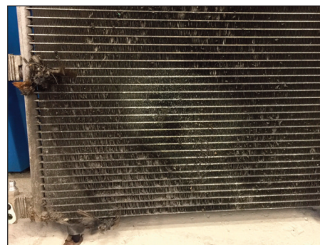
It may not leak, but this condenser cannot perform well and must definitely be replaced
