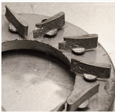
Hardened particles inside the exhaust system have continuously impacted and damaged these variable guiding vanes
