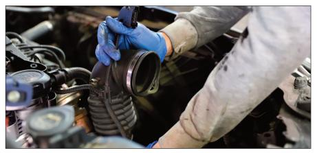
Impaired tightness of the ducts that channel air within the turbo circuit is one of the major problems affecting the turbocharged system's functionality.
