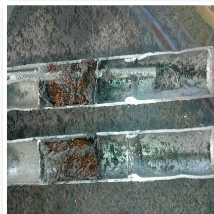
Worn out desiccant and filtering layers inside the receiver dryer
