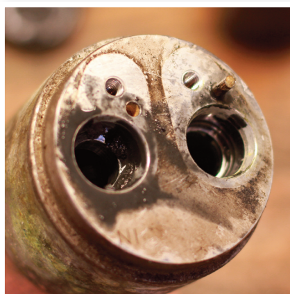
Contamination of the inlet or outlet will cause the receiver dryer to clog
