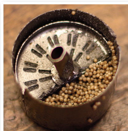
The desiccant layer inside this receiver dryer is overflowing
