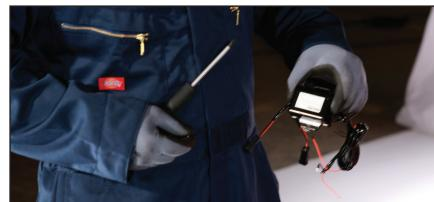
3) Find a solid place under the bonnet to mount the control box, (preferably near the battery and away from heat). Don't fix box yet, but ensure the mounting surface is clean.
