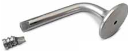
Fig. 1: forced breakage at groove
