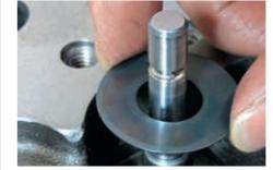
Oil the valve stems before final mounting and insert the valves into the valve guides. Fit the valve spring seats or the valve rotators (if prescribed).
