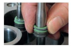
Slide the valve stem seals over the valve stems using an oiled protective bushing.
