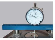
The valve recess dimension must correspond to the manufacturer's specifications (repair shop manual). If the valve recess is too great, the valve must be replaced. If the valve recess is too small, check whether the correct valve is being used. Replace the valve if required, or rework the valve seat insert until the prescribed recess dimension is achieved.
