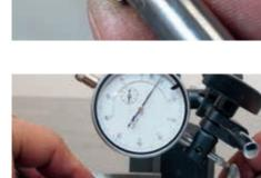
Concentricity of the valve seat surface must be checked using prism and dial gauge. Bent valves must always be replaced.
