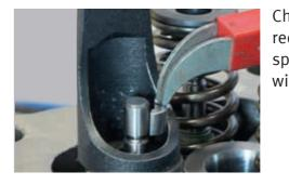
Check the valve springs for length and rectangularity. Insert valve springs with valve spring retainers and press down valve cotters with a suitable tool or equipment for mounting.
