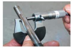
The valve shafts must not exhibit any visible wear.
