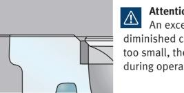
Attention: An excessively large valve recess leads to diminished compression. If the valve recess is too small, the valve may collide with the piston during operation.
