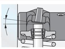
Used rocker arms must not be bent or torn. Oil bores for lubricating the rocker arm and rocker arm shaft must be unrestricted.
