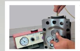
The required check for valve tightness can be performed by means of a vacuum test from the duct side. Alternatively, the combustion chamber bowl can be filled with a small amount of fluid (petrol, petroleum).
