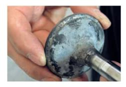
The valve seats on the valves must not be staved in. If they are: Replace valves or rework valve seats using a valve grinding machine.
