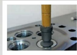
If there is a leak, first check the valves for radial eccentricities and damage before reworking the valve seat inserts or grinding in the valves.
