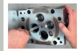
De-wax and wash new cylinder heads and check for external damage. Clean oil bores and valve guides with a brush.
