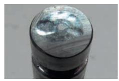
The valve stem faces must also not be damaged. Therefore rework damaged valve stem face surfaces or replace valves.
