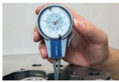
The diameter dimensions of the valve stem and valve guide are deducted from each other and compared with the clearance specifications of the manufacturer. If the clearance is too great, the valve may be worn and must be replaced. If the clearance is too small, then the valve guide must be reworked using a reamer.
