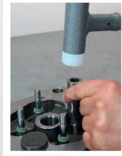
Push the valve stem seals onto the guides using a suitable fitting tool. Valve stem seals with a plastic supporting body
