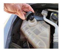
A common cause of engine overheating is a faulty pressure relief valve in the radiator cap. If this is contaminated, the engine cooling system may be impacted. A simple measurement of the temperatures in the cooling system, will quickly indicate whether the radiator cap is the root of the problem. If the temperature is OK, take a closer look at the entire cooling system. If you find that the radiator cap is faulty, replacing or cleaning it, may be enough to rectify the problem.
