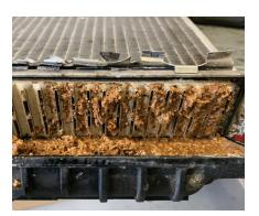
If it is determined that the radiator is no longer effectively dissipating heat, flushing the radiator can help remove minor blockages. Dirt or deposits can block the cooling fins, which significantly impairs the cooling performance. However, if cleaning is not sufficient, e.g. because the fins are bent or scale has formed inside the radiator, it is often necessary to replace the radiator. Even if the coolant level is too low or the coolant is incorrectly dosed, this can lead to overheating.
