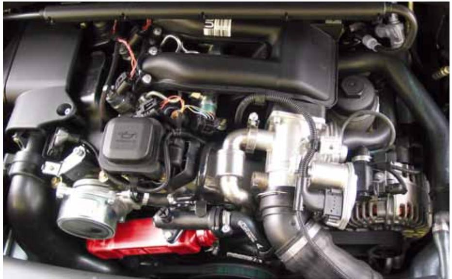
Fig. 2: EGR cooler in a BMW 318d (highlighted in red)
