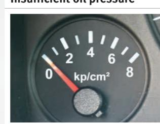
Insufficient oil pressure leads to premature wear of the bearings or to bearing damage. The main reasons for this are:
