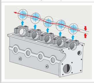
If the centre points of all main bearing points are not exactly central on an axis, severe bearing damage occurs when starting due to the necessary bearing clearance being eliminated. Such problems are caused by bent or incorrectly ground crankshafts and a distorted engine case (previous damage caused by overheating).
