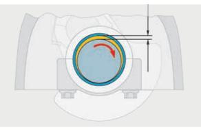
The bearing clearance ensures that in every operating situation there is sufficient space between the bearing and the bearing journal. This enables a strong and
