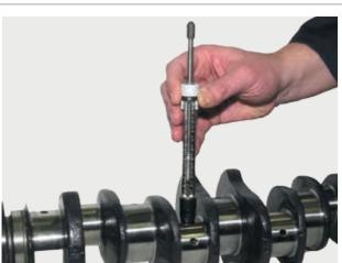
As a result of bearing damage (overheating of the bearing points) shaft journals regularly lose the necessary hardness.
