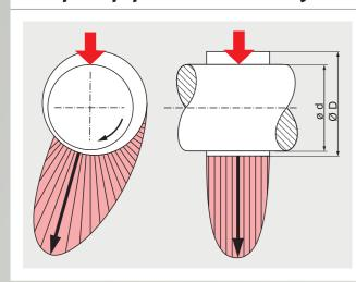
The oil pump pressure generated by the oil pump has the function of conveying the oil to the bearing point and cooling the bearing by a constant flow of oil.
