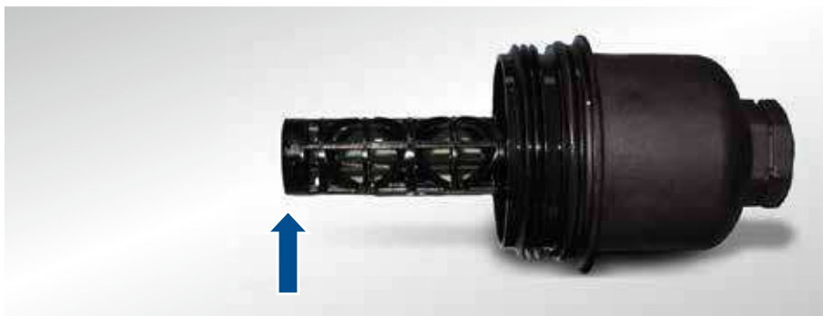
Fig. 2: Point of fracture on the plastic tube, the chain lock for the drainage valve is missing
