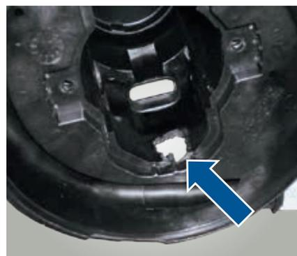
*Damage: melting traces on the housing (top view into the housing)*
