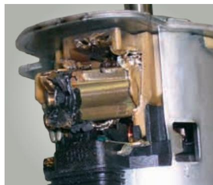
*Damage symptoms: melting traces on the electric motor or on the electrical contacts*
