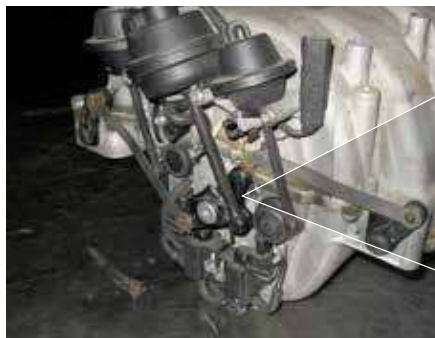
Damage symptoms: Fracture on cam control mechanism
