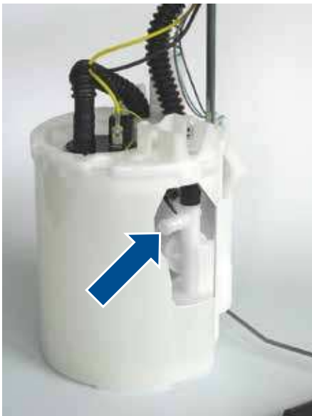
Fig. 1: View into the fuel delivery module (cut-away view) with blind-mate connector
