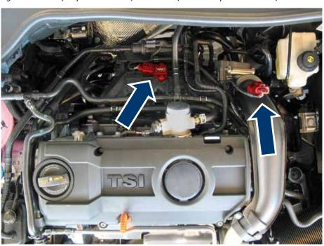
Fig. 2 Intake manifold pressure sensors (red) in a VW Golf IV
