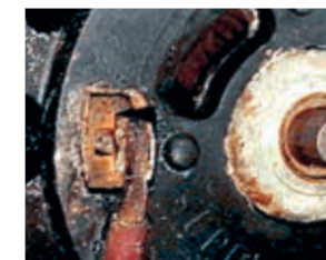
Secondary air pump – corroded electrical connections
