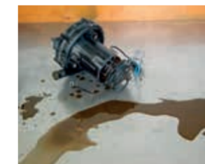
Condensate in secondary air pump
