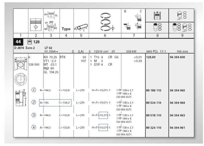
Fig. 3: Non-binding extract from the KS catalogue "Pistons/Cylinders/Kit sets"
