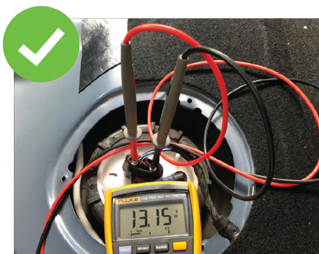
Fig. 1: Voltage is checked at the cover of the fuel delivery module
