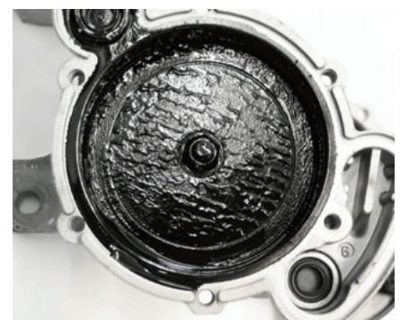
Fig. 3: Oil sludge in the vacuum pump of the VW Transporter results in rattling noises
