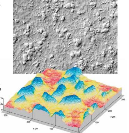
3-D roughness record of a finished ALUSIL® cylinder sliding surface
