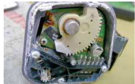
View of the interior of a damaged regulating throttle
