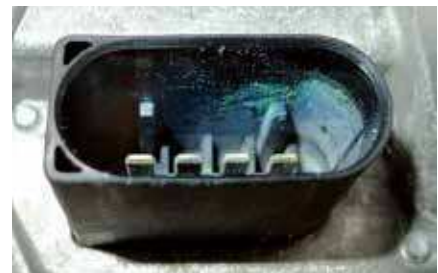
Built-in plug with traces of corrosion
