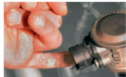
*Finger check at secondary-air valve in BMW 520i (highlighted)
