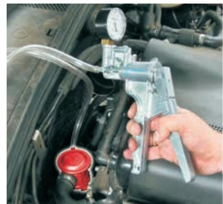
*Checking a secondary-air valve with a vacuum hand pump*
