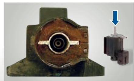
*Corroded solenoid switching valve (open)*
