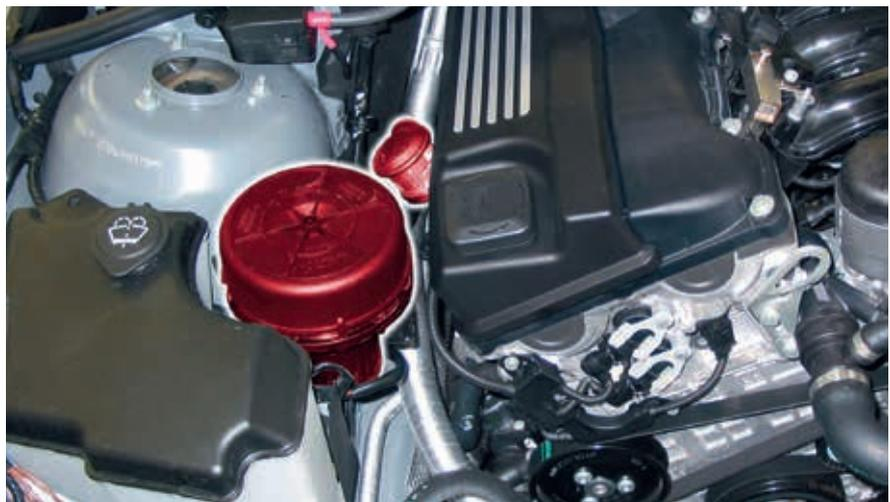
Secondary-air valve and secondary-air pump in BMW E46 (highlighted)
