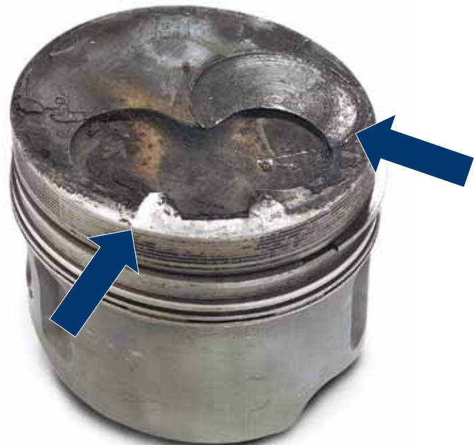
Fig. 4: impact marks due to engine overheating
