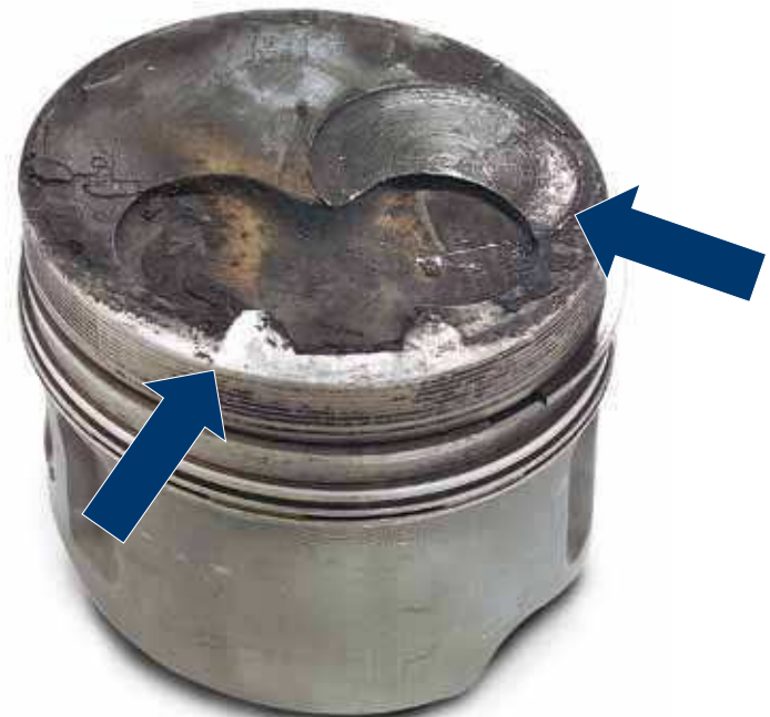
Fig. 4: impact marks due to engine overheating
