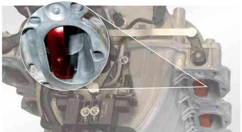
Tumble flaps (highlighted in red) in the PIERBURG intake manifold, e.g. in the Mercedes E-Class 500
