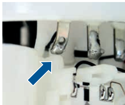
Fig. 2: The cable is pulled off if the compression of the fuel delivery module is too extreme.
