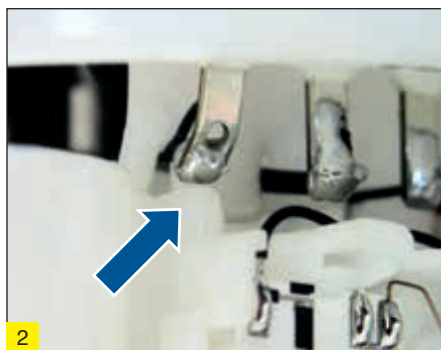
2 The wiring is pulled off the connection if the compression of the fuel delivery module is too extreme
