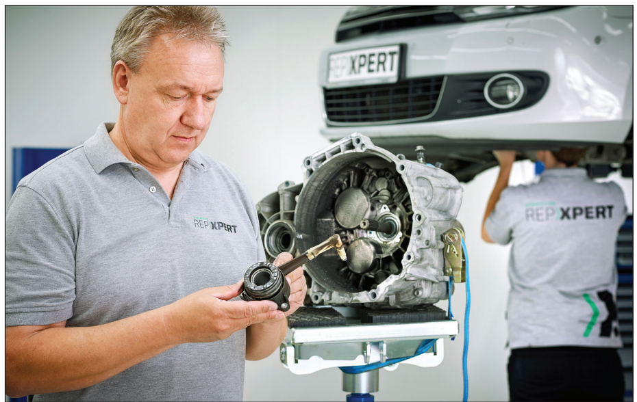
REXPERT Trainer Ralf Kuhlmeiy recommends to always replace the CSC when servicing a clutch
