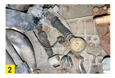
battery tray, and then the engine ECU. This gives good access to the top of the gearbox (Fig 2). Remove the engine speed sensor from the back of the bellhousing, disconnect the reverse light switch, gearbox earth strap, then disconnect both gear change cables and cable bracket, and stow them out of the way. Remove the upper bellhousing and starter motor bolts, then fit the engine support, if a bridge system is being used.
