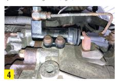
pipe bracket bolt. Ease the slave cylinder away from the gearbox, and remove the air charge cooler pipe that runs under the engine/ gearbox. Detach the lower gearbox pendulum mounting and retaining bracket, as well as the tin cover plate at the bottom of the bellhousing. Remove the lower bellhousing bolts, leaving a couple of easily accessible bolts to support the gearbox until the point of removal, lower the lift to waist height and
