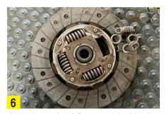
This spring can break from excess load/hard driving or vibration, from an engine misfire for example, being transmitted through the clutch, causing the springs to fully compress and then break.
