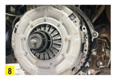
Clean the new clutch pressure plate with clutch and brake dust cleaner, to ensure the face is degreased and, using a clutch alignment tool, mount the new clutch (Fig 8). Tighten the bolts in an even and sequential manner and then torque to the
