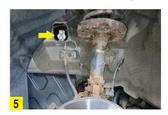
remove the two gearbox mounting bolts that are accessed through the inner wing (Fig 5), then lower the lift and remove the mounting from the gearbox. Raise the lift to gain access to the underside, support the gearbox with a transmission jack and remove the final bellhousing bolts. Ease the gearbox away from the engine. When the gearbox input shaft is clear of the clutch, lower the gearbox, remove the gearbox from the vehicle and place it somewhere safe.
