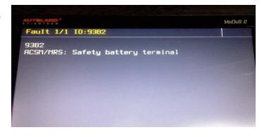
terminal. With this information, we were confident that replacing the safety battery terminal would cure the fault. The safety battery terminal was replaced and the fault was cleared, and didn't return.
