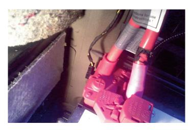
Most modern BMWs have a safety battery terminal. The air bag control module fires a pyrotechnical device within the terminal that disconnects the battery when a collision occurs.
