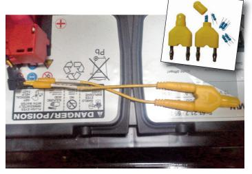
A test lead from the ATA95 Test Lead Kit (inset) holds a resistor to mimic the safety battery terminal. This allowed the rest of the circuit to be tested, narrowing the fault to the battey terminal itself.
