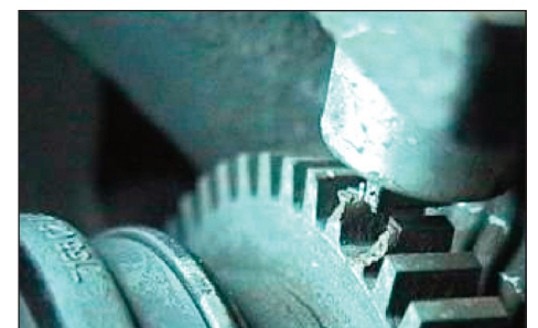
Figure 3: Defective teeth on the ABS disk were good enough for lower speeds
