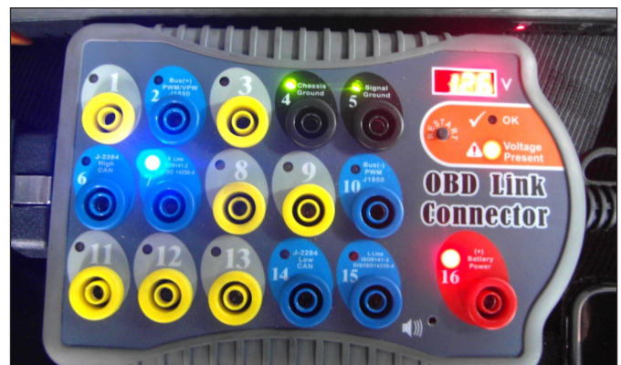
Fig. 2 The light at pin 7 on the DLC Breakout Box indicated a fault in the K-Line. A scope could also be used to see the signal at any pin.
