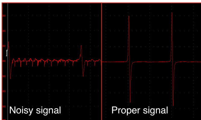
Fig. 1 The noisy crank sensor signal on the left, and a proper, clean crank sensor signal on the right.
