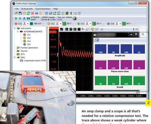
the scope software. Switch on the current clamp and zero out the current clamp. Start the measurement by pressing the start button or the hotkey S. Crank the engine for 2 to 4 seconds to record the current data. The relative compression test is now ready and will look like figure 2.
